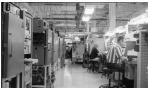
Sensotec transducers undergo extensive environmental testing during manufacture.
