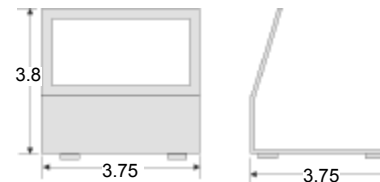
AA944 Bench Mount Kit for 1/8 DIN
