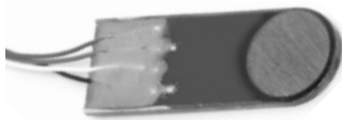
The original patented miniature pressure transducer.
